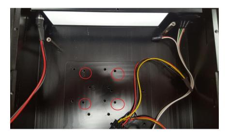
3./ Use the screw holes on the thermal module, as the illustration below shows with the inlet on the thermal module facing the rear of the chassis.
